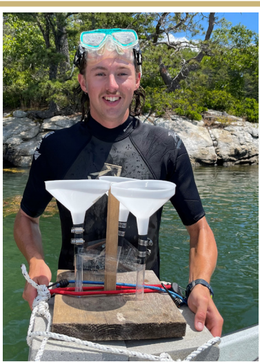
Peter Dunbar, Bates rising senior, displays the experimental sediment traps he designed to determine how much sediment accumulates on the bottom of a given area over time. These unique measuring devices, which are secured by cement blocks, have been sunk at our sites at both Denny Reed and Thistle Point in the Basin. This experiment and its results will be the basis for Peter’s senior thesis.
